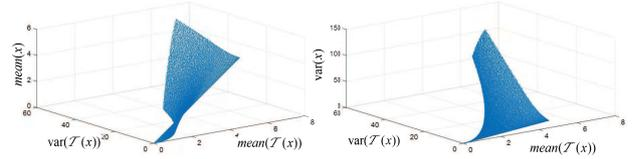
Figure 4. 2D look-up tables for correcting the clipping effect of  $\text{mean}(\cdot)$  (left) and  $\text{var}(\cdot)$  (right).
